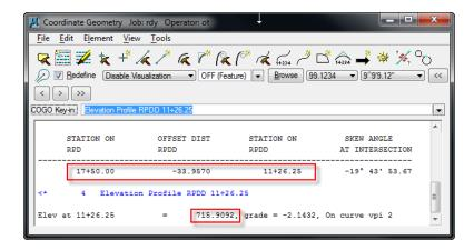
If the cross sections are cut using the default DTM's and about -RPD- alignment, then profile elevation of the offsetting -RPDD- alignment is off (0.2798' or  $\sim$ 3.36").
