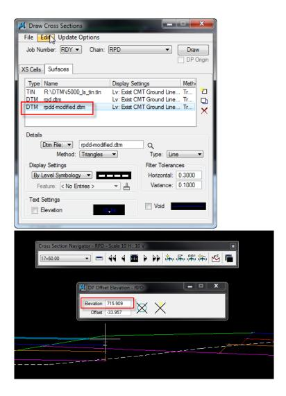
Of course this will tie down the offsetting corridor profile elevation. Since the whole -RPDD- surface DTM is just an interpolation of data between two template drops, the other Important tie point(s) like to the existing ground is still "skewed". This will have to be modified manually this in the XSC.
